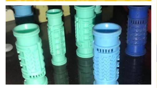
A Multi Cavity Mould has been designed, developed and manufactured for drip irrigation system. These components are being used for optimum drip watering for tea plantation for optimal water resource utilization.
